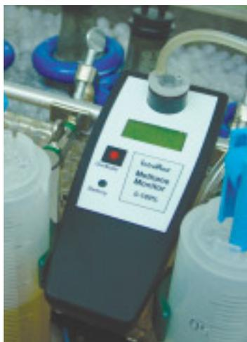
Laboratory bioreactors (top) provide accurate measures of the bioenergy content in various composting feedstocks. The methane monitor (bottom) provides readings from the bioreactor units.
