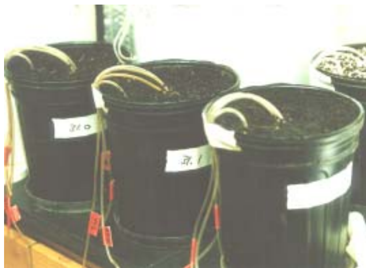
Figure 1 Oxygen measuring lines inserted container-media into pots at varying depths.
